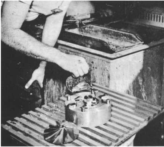
Molten alloy is dipped from holding tank in rear and poured into a jig around the rotor being invested for machining- Note easy, safe handling of low-temperature-melting alloy.
