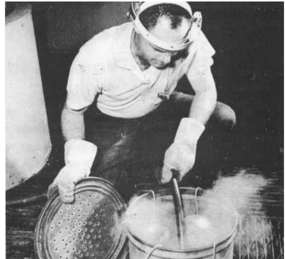
Removal of the alloy is accomplished here by steam line discharging into an ordinary steel bucket- Removal could also be done by hot water bath. Individual parts come clean, with only slight hand scouring in the case of anodized aluminum rotors. Lighter metal chips float on molten alloy which is then reclaimed for reuse.
